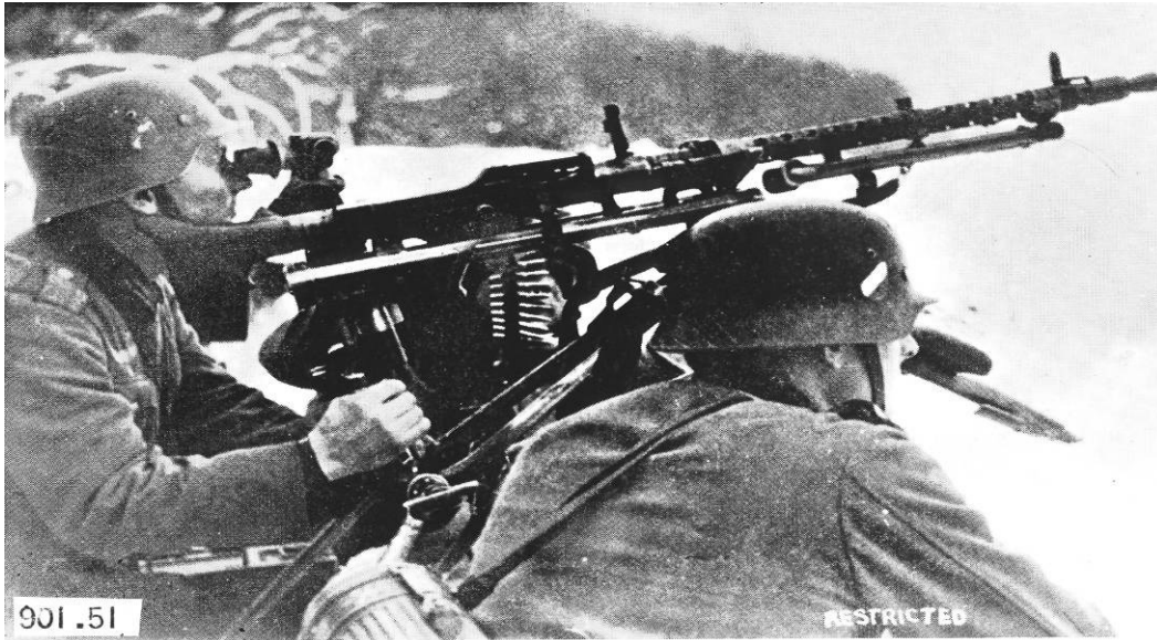
PLATE 9.—M.G. 34 on Heavy Mounting. Note the dial sight with which this weapon is equipped.
